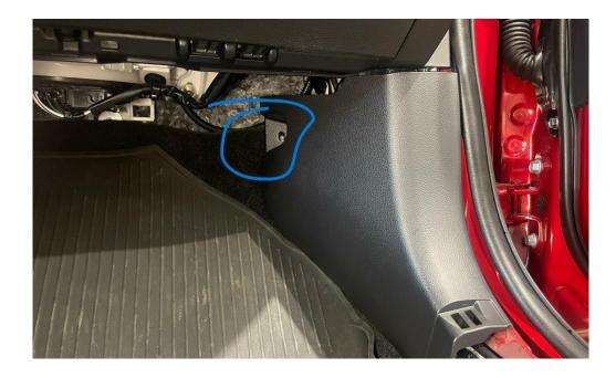
**17.** Unlink the glove box from the side and squeeze the inside of the box to allow the plastic arm to move out of the dash. Lower the glove box all the way down then it can be removed, try different angles if needed, and don't use force to pull it out.
