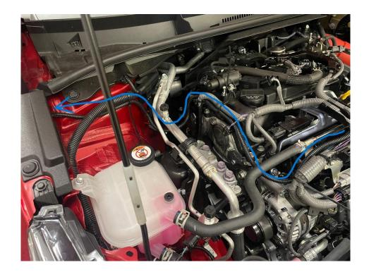
**12.** Feed the wire into the wheel well, it will need to be passed through from an existing hole on the passenger side behind the fender liner. Lift that side of the car and remove the wheel, remove the backside of the fender liner, and secure the wire using the OE bracket.
