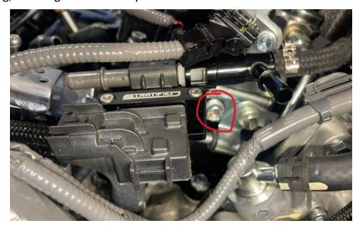
**8.** For the fuel line connection, start from the HPFP to connect the longer custom fuel line, push in until it clicks. Rotate the T fitting towards the OEM fuel quick-disconnect connector, guide it under the wiring harness, and connect to the ethanol sensor first, then push in the OEM quick-disconnect connector and press down on the orange plastic tab to lock it.
