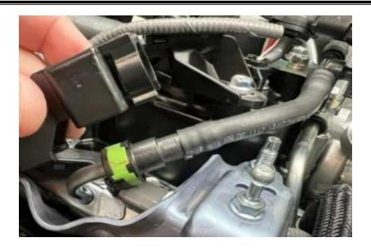
**6.** Locate the bolt that secures the OE T fitting from the bottom, and remove with a 10 mm socket. This OEM fuel line with T fitting will be replaced with our Stratified custom lines, so store it in case of reverting back to the OEM fuel line setup. We will still use the same bolt and location to secure the ethanol sensor.
